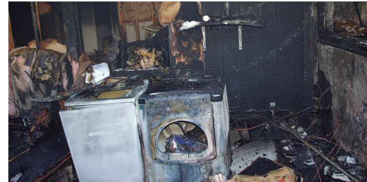
Photo courtesy of the Menlo Park Fire Protection District. This photo shows the washing machine where the fire originated.
